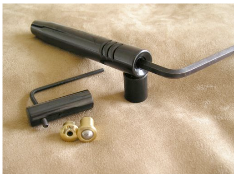
Picture 1: To remove the muzzle plug with the Allen key provided (1/4"), the front fixing bolt, that retains the brake catch to the body, must be removed. A 3mm key is required. The refitting is aided by a secondary location peg, which helps realignment. Also shown are countersunk fixing (std) and alternative ball bearing fixing. It is important to keep the threads of both muzzle plug and brake body free of any contamination. The muzzle plug is only partially broached to accept the Allen key. Apply forward pressure to the Allen key as it is used to screw and unscrew the muzzle plug to prevent "rounding off" the hexagonal internal broach.
