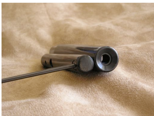
Picture 1: In order to remove the muzzle plug with the Allen key provided (1/4"), the front fixing bolt, that retains the brake catch to the body, must be removed. The 2 nd fixing bolt can be slackened to allow the catch to separate slightly from the brake body. It is important to keep the threads of both muzzle plug and brake body free of any contamination. The muzzle plug is only partially broached to accept the Allen key. Apply forward pressure to the Allen key as it is used to screw and unscrew the muzzle plug to prevent "rounding off" the hexagonal internal broach.
