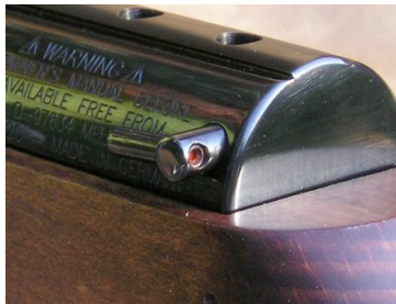
Picture shows RS Safety Catch depressed and rifle ready to fire.
