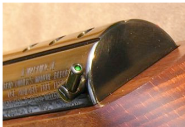
Picture shows RS Safety Catch reset after Mode 1.
